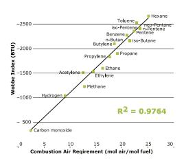
The table and graph above show the relationship of Wobbe Index and the Stochiometric Dry Air Requirement for some typical gas constituents. The correlation is close to linear (R²=0.9767) with an intercept close to zero. The residual oxygen method takes advantage of this correlation by linear extrapolation between measurements of known calibration gases. R² for typical natural gas constituents plus hydrogen and CO is 0.9888.
